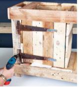
**5** Place the 390mm plank at a right angle across the middle of the four 420mm planks and screw down in a zig-zag pattern. Turn the door over and attach two hinges to the front. Now attach the door to the frame and fit a handle.
